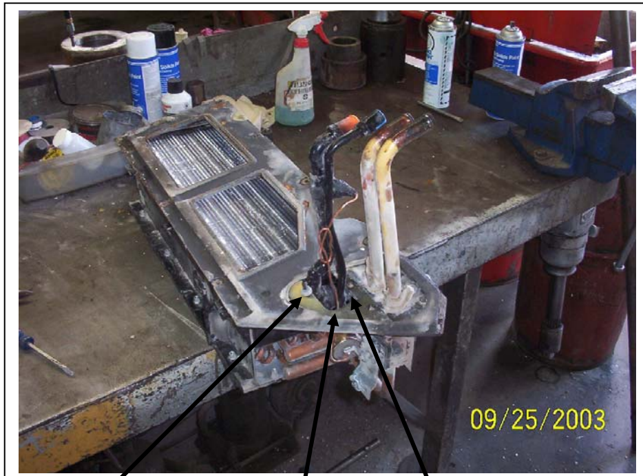
Reused nipple for the windshield washer hose.
