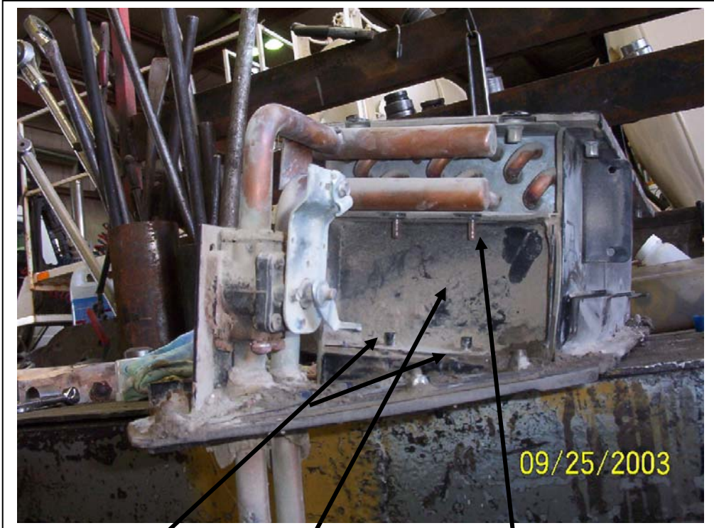
Locator pins on box. Trim these two off to 1/8" long to clear the suction header pipe.
