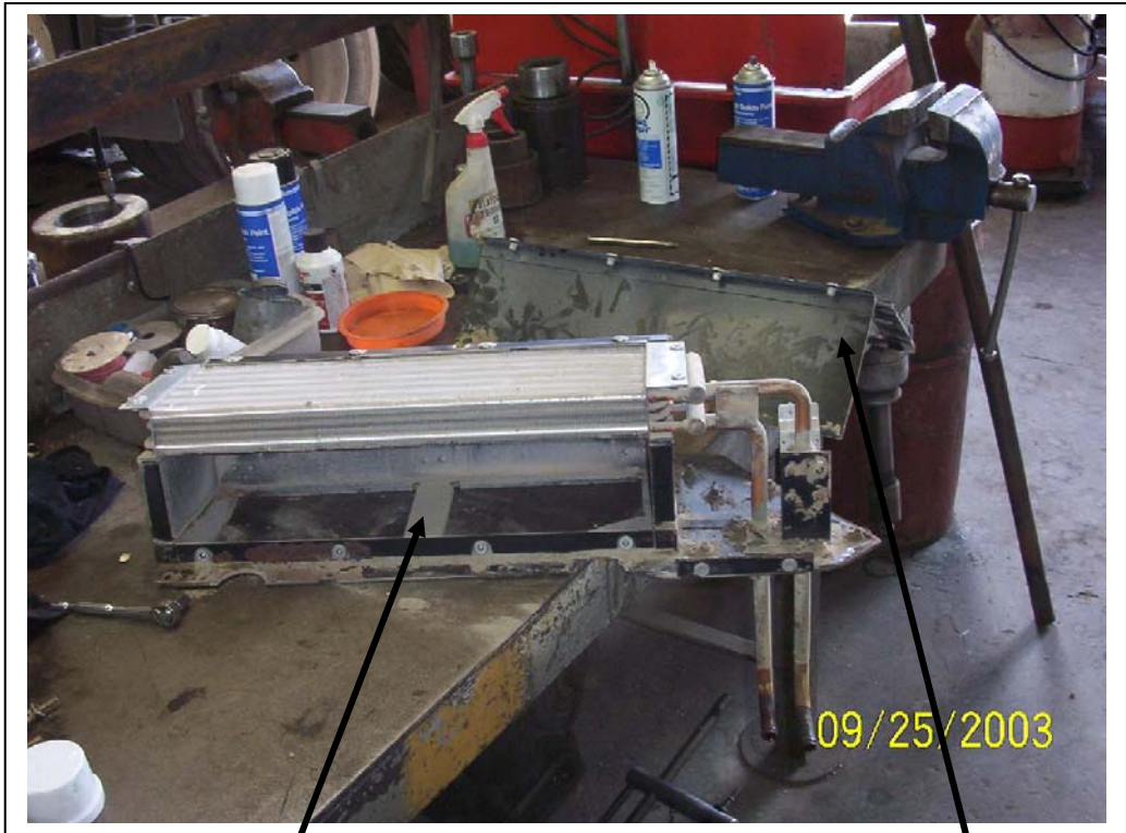
Heater box removed from cab Heater box lid
