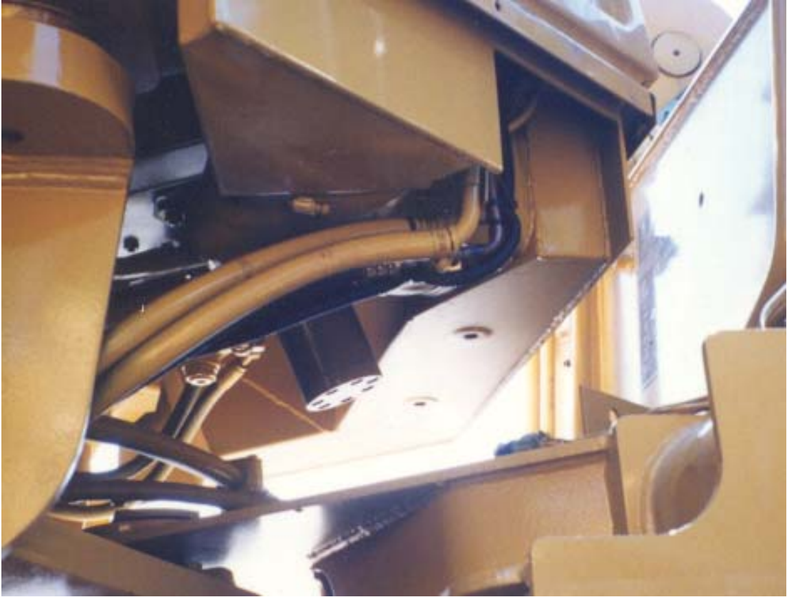
Hoses under cab.
