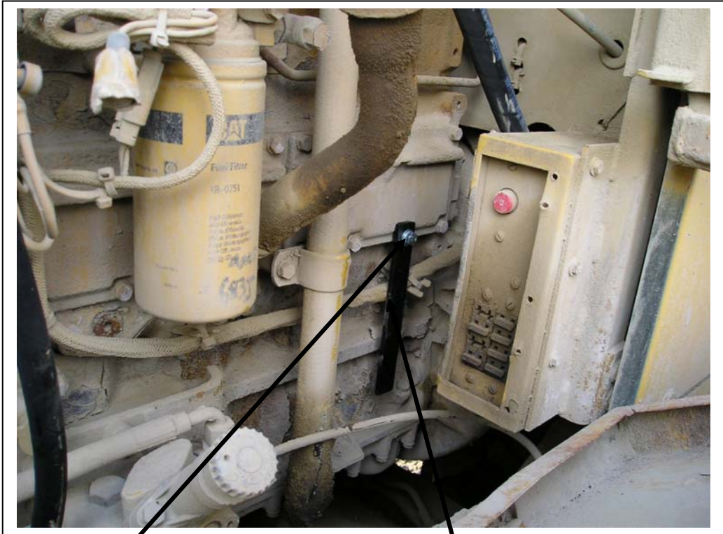
M8 bolt and 1/4" thick spacer behind mount bracket.
